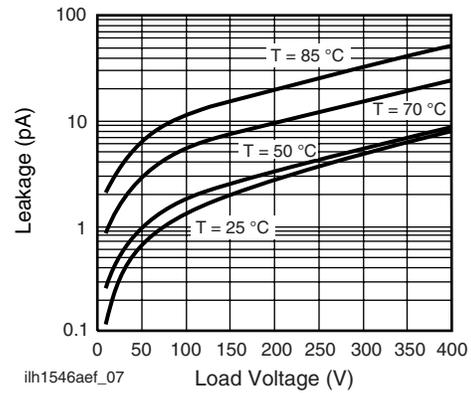
Fig. 6 - Leakage Current vs. Applied Voltage
