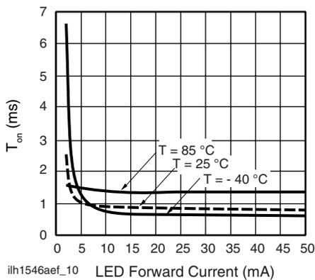
Fig. 9 - Turn-on Time vs. LED Current
