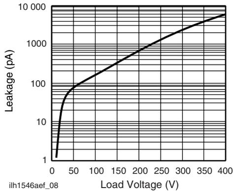
Fig. 7 - Leakage Current vs. Applied Voltage
